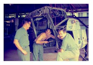
Remember, these Aussies had no Birddogs in their inventory or the corresponding access to jigs, templets, or instructions on how to put one back together. Damaged skin panels from one wreck were flattened out to use as templates. New panels were hand-cut and drilled. Many items were 'donated' by US Army Aviation. How the tail-wheel assembly was acquired, demonstrated the lengths 161 Possums were prepared to go:
