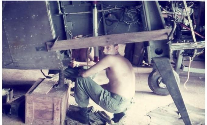
**Sgt Zitzelsberger and L/Cpl Bower working on fuselage alignment. Note the creative rigging and alignment “tools” in use.**
